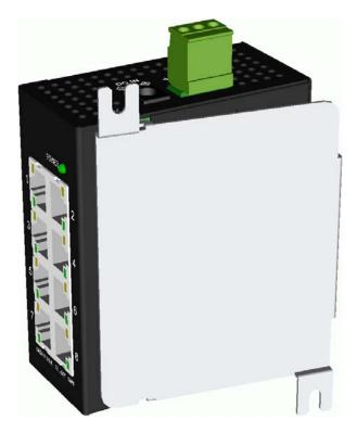
2. Screw the bracket on the switch unit.
