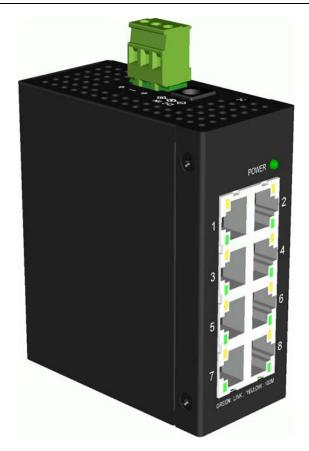
The switch provides eight 10/100Mbps copper ports for connections to Ethernet and Fast Ethernet devices. With the featured auto-negotiation function, the switch can detect and configure the connection speed and duplex automatically. The switch also provides auto MDI/MDI-X function, which can detect the connected cable and switch the transmission wire pair and receiving pair automatically. This auto-crossover function can simplify the type of network cables used.
